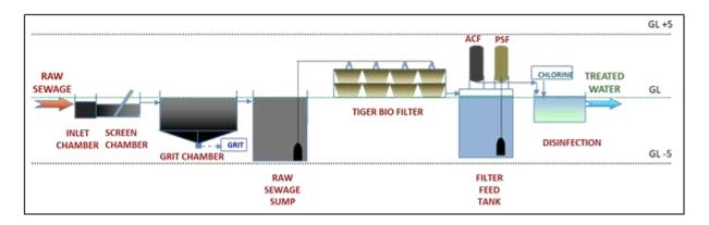
The Tiger worms used are the species capable of compositing human waste rapidly. The system is designed accordingly with sufficient surface area and worm quantity. The worms consume the sewage organic load in 24 Hrs making bed available for next day loading. As the worm population is self-regulating depending upon availability of food (organics) resulting in increased efficiency and operational feasibility.
